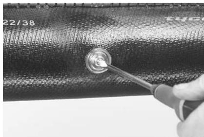
**26** Insert the valve plug or other device.
