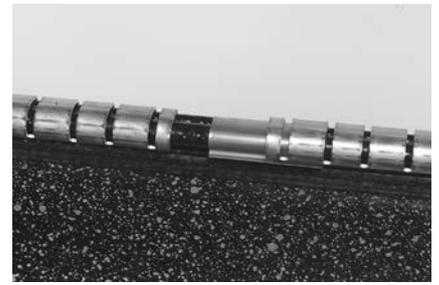
**15** Slide the flexible channels over the sleeve rails leaving a small gap at the center for the retention clip. Position the retention clip in the opening between the channels and slide the channels evenly over the clip.
