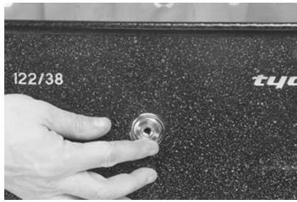
**14** Attach the sleeve to the canister with the valve nut and hand tighten.
